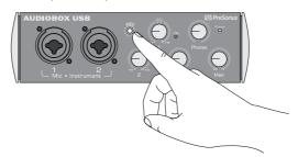
Turn up the Channel 1 level on the AudioBox USB while the ensemble is playing the loudest it will be performing. You should see the input meter in Studio One Artist react to the input.
