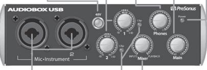
Microphone / Instrument Inputs. Each input channel has both a microphone and an instrument preamplifier. The combo connectors allow you to use either a ¼" TS or the included XLR cables. Use the ¼" connection for guitars and other unamplified instruments. Use the XLR connections to connect your PS626 microphones.
