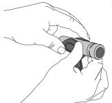
To assemble your stereo bar, begin by removing both microphone clips and positioning each clip at a 90° angle to its yoke.
